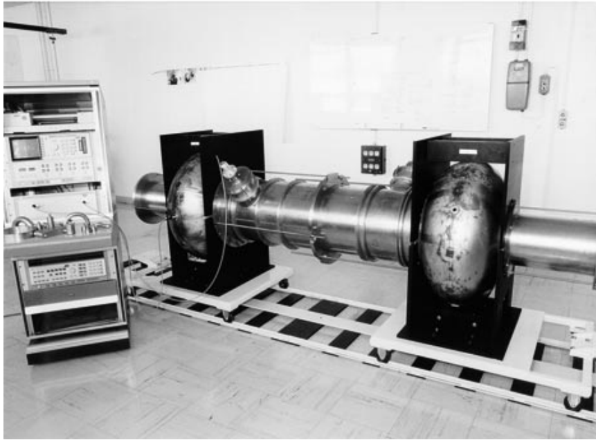
Figure 4 : The copper assembly used for the damping optimization
