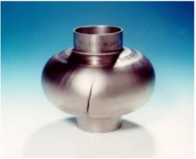
Figure 7: Nb RRR 20: rupture at 208% expension (instead of 216%)
