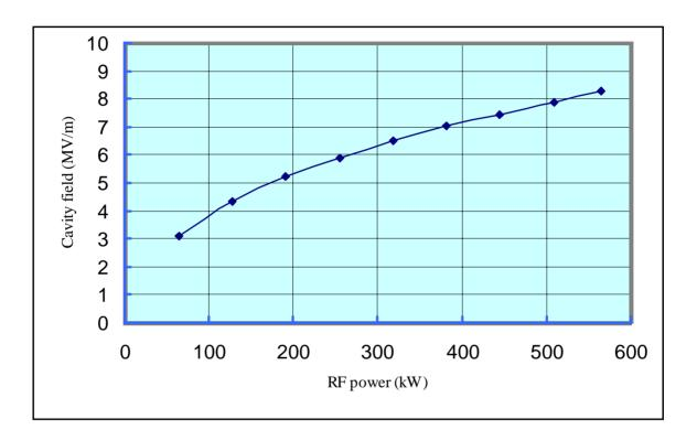
Figure 3 Cavity field versus RF power
