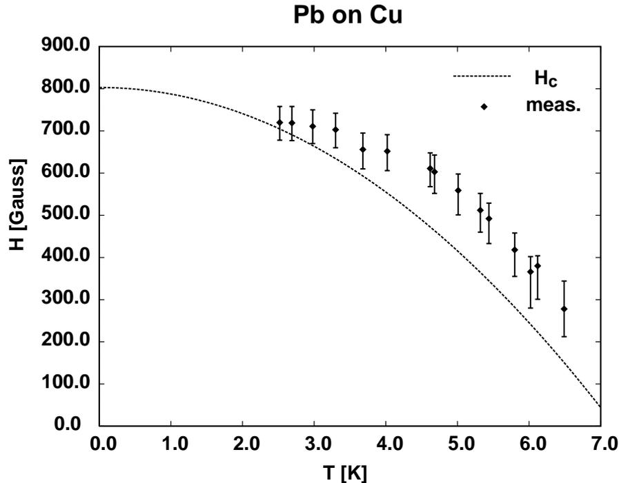
Figure 3: Measuring the  $H_c^{\text{rf}}$  of lead by pulsing a lead coated copper 1.3 GHz cavity.
