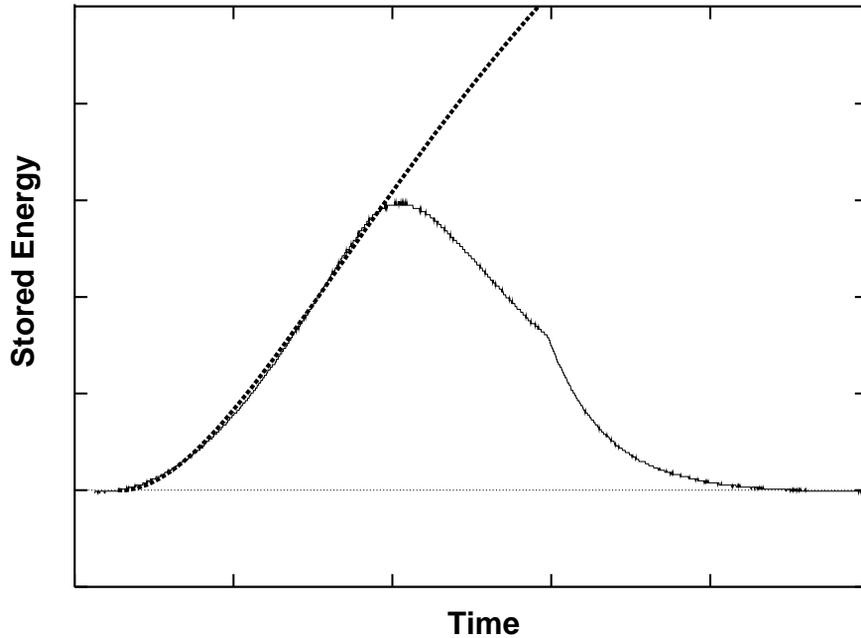
Figure 1: Comparing the behavior of a cavity that quenches with an idealized cavity with no quench. The point where the two diverge is the  $H_c^{\text{rf}}$ .
