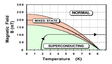
Figure 1 - Phase diagram of niobium giving the critical magnetic fields  $(B_1, B_2, B_3)$  as a function of temperature.
