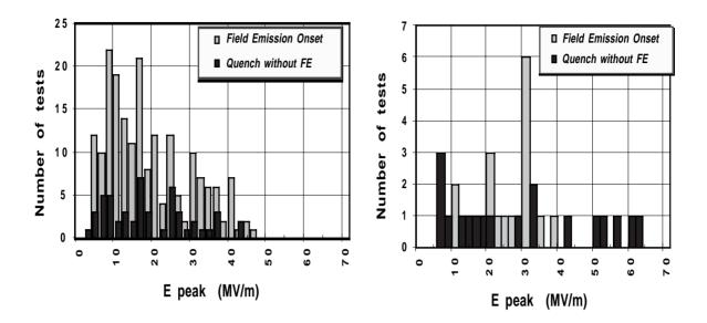
Figures 6a & 6b- Field emission thresholds statistics on 320 tests performed at Saclay before and after January 1996. Cavities without FE are now obtained with peak fields exceeding 60 MV/m.
