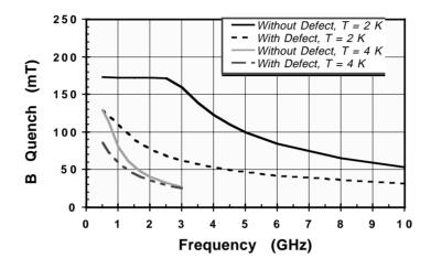
Figure 3 - Calculated quench field value with and without defect as a function of frequency for a RRR 250 niobium cavity and helium bath in the superfluid state (T = 2 K) and normal state (T = 4 K).
