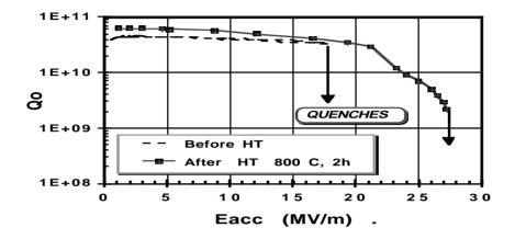
Figure 5 - The cavity C110 made from niobium RRR 400 sheets improved its quench field after only a  $800^{\circ}$ C, 2 hours annealing.
