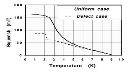
Figure 2 - Calculated quench field value for a niobium RRR 200 cavity, thickness 2.5 mm at a frequency of 1300 MHz in the uniform case and in the case of a normal defect (size = 20  $\mu$ m,  $\sigma$  = 10  $^{7}$   $\Omega$   $^{-1}$ .m  $^{-1}$ ).
