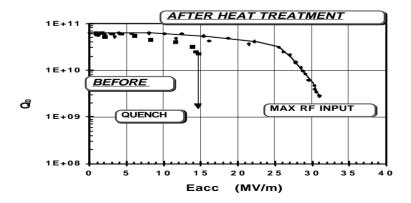
Figure 4 - Single-cell cavity C101 (initial RRR 250), quenching at 15 MV/m before heat treatment. The improvement after heat treatment is impressive (> 31 MV/m without quench).
