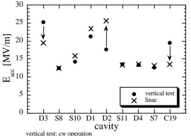
linac:  $305 \,\mu\text{s}$  rise time,  $800 \,\mu\text{s}$  constant gradient at  $10 \,\text{Hz}$  rep. rate
