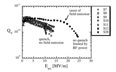
Fig. 4: RF-performance of cavities produced by one manufacturer with old (S7 to S12) and improved (S28) welding technique.
