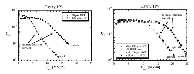
Fig. 6: RF performance of the first 1.3 GHz single-cell cavities made by spinning.
