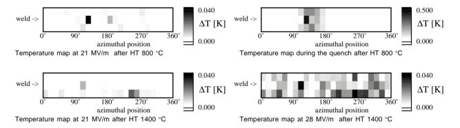
Fig. 5: Temperature maps of equator region of cell 9 of cavity C21 at different field levels and after heat-treatment (HT) 800 °C as well as after HT 1400 °C. The distance between thermometers on the weld and below or above the weld is 1.2 cm, the azimuthal distance is 2.5 cm. Note the strong reduction of heating after the HT 1400 °C.
