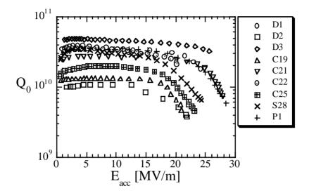
Fig. 1: Vertical test results on 9 cell cavities for the TESLA test facility linac. C21, C25, S28 and P1 are limited by field emission and available RF power. The other cavities are limited by quench.
