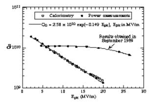
Figure 3:  $Q_0$  versus  $E_{pk}$  of a cavity heat treated at very high temperatures. Both (conventional) rf power measurements and results from the thermometry system are included. For comparison, results from 1989, where no Q-degradation was observed, are also depicted.
