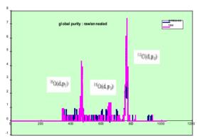
Figure 8: Comparison of O and C contamination between raw and annealed niobium (mean values)
