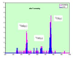
Figure 9: Comparison of O and C contamination between grain and boundaries for annealed niobium (mean values)
