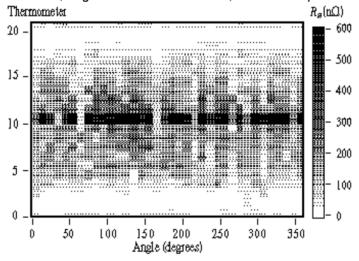
Figure 4: "Flattened" surface resistance map of one of the heat-treated cavities, as deduced by thermometry. The equator is at thermometer #10, and is characterized by a dark band because the cavity is thinner along the weld. The irises are at thermometers #1 and #19. For reference: A cavity with  $Q_0 = 10^{10}$  should have a surface resistance of about 27 n $\Omega$ .
