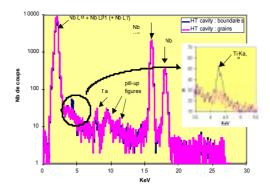
Figure 5: PIXE spectra for cavities samples.
