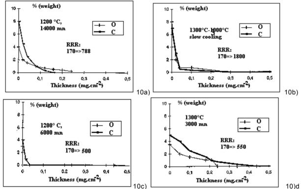
Figure 10 : profile concentration of oxygen and carbon for four different annealing conditions, along with RRR measurement.
