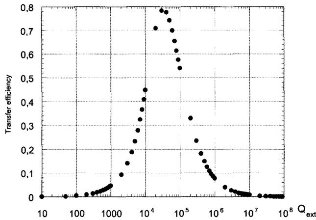
**Fig. 2 - Transfer efficiency versus external quality factor for out pulse length (4.5µs)**
