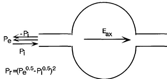
Fig. 1 - Powers and field in the cavity
