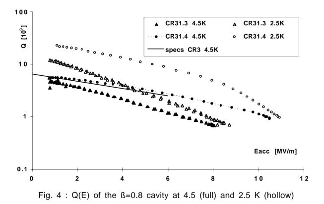
It was realized that the magnets used to coat the cut off tubes were not optimally positioned, resulting in a grazing angle incidence on the cavity side wall. This has been corrected in the fourth coating. The cold test showed a Q(E)
