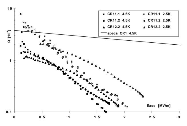
Fig. 2: Q(E) of the two ß=0.48 cavities at 4.5 K (full) and 2.5 K (open)
