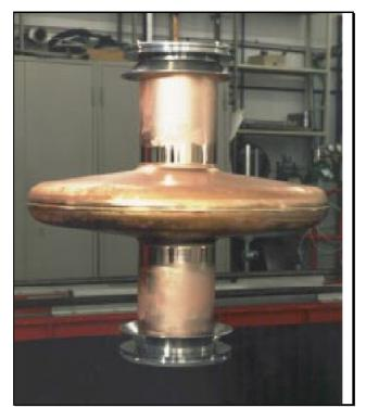
Photo: Copper cavity  $\beta$ =0.48 ready for sputtering
