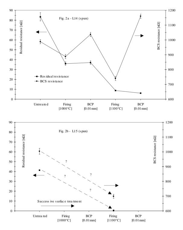
Fig. 2a-b : Effect of surface treatments of spun cavities on  $R_{res}$  and  $R_{BCS}$ . Cavity L15 (bottom) has been fired only at 1100°C, therefore no data at 1000°C are available. Small errors are included in the data points.
