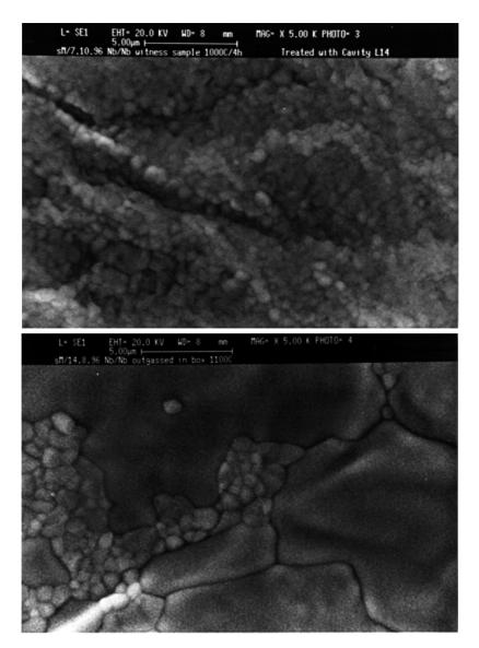
Fig 4. : SE-micrographs showing the structure of the film at  $1000^{\circ}$ C (top) and when anomalous grain growth appears (bottom).
