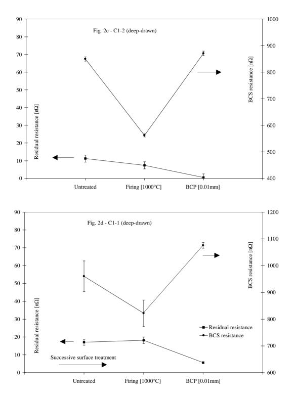
Fig. 2c-d : Effect of surface treatments of deep-drawn cavities on  $\rm R_{_{res}}$  and  $\rm R_{_{BCS}}$
