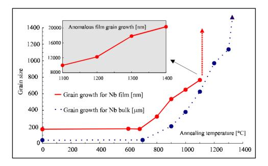
Fig 3.: Evolution of the grain size of the substrate and of the film (1.5 $\mu$ m) as a function of the temperature of thermal treatment.
