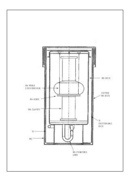
Figure 1: Schematic view of a cavity enclosed in a protection/gettering set-up
