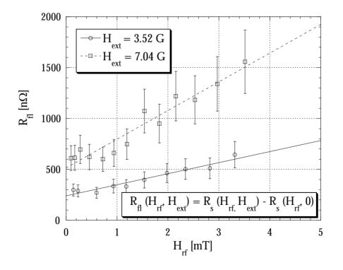
Fig. 7: Variation of the contribution induced by  $H_{ext}$  to the surface resistance of the resonator, as a function of the RF field  $H_{rf}$  for T = 4.2 K. The displayed fit is of the form:  $R_{fl} = (H_{ext} - H_{th})(R_{fl}^0 + R_{fl}^1H_{rf})$ .
