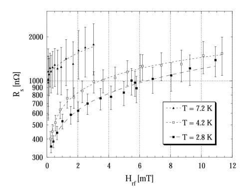
Fig. 5: Surface resistance of the 1.5 GHz NbTiN/Cu cavity as a function of the RF field at different temperatures.  $E_{acc} = 1 \text{ MV/m}$  corresponds to  $H_{rf} = 4.55 \text{ mT}$ .
