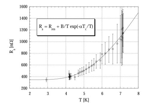
Fig. 6: Variation of the surface resistance as a function of temperature for  $H_{rf} = 0.23$  mT. From the displayed fit, putting  $T_c = 14.2$  K, one gets  $R_{res} = 350$  n $\Omega$  and  $\alpha = 2.3$ .
