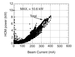
Figure 7: The HOM power absorbed by the dampers.
