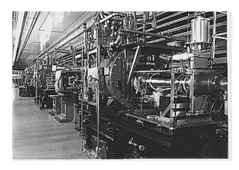
Figure 10: Four SC damped cavities installed in HER.
