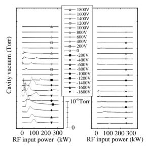
Figure 8: Mapping of vacuum pressure versus input power, scanning the power for the various bias voltages up to  $\pm 1.8 \text{kV}$ .
