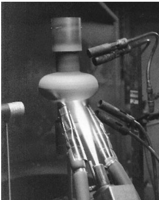
Figure 3 : HVOF spray of a monocell 1.3 GHz cavity
