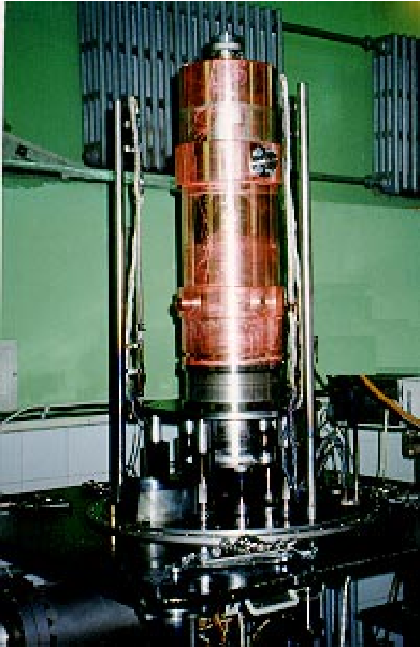
Figure 1: The QWR installed on the supporting frame.
