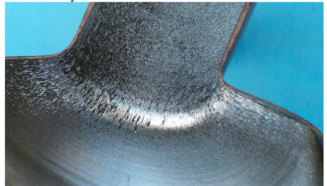
Fig. 11 – Section of a Nb clad Cu cavity after vacuum annealing. Pre-existing cracks at the iris due to the material tensile strength at the time of spinning were amplified by the different thermal expansions of Copper and Niobium.
