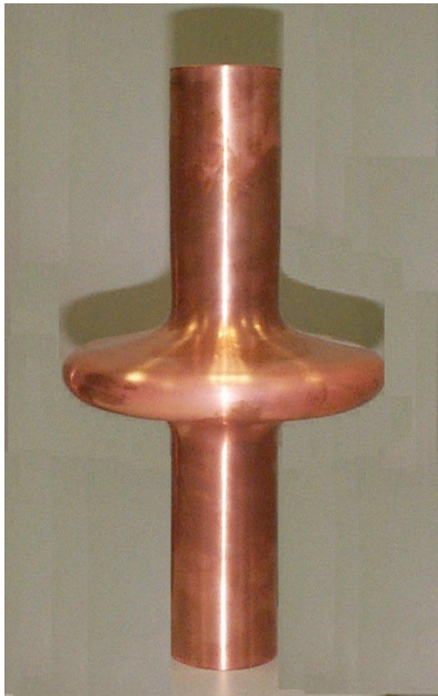
Fig. 2 - A beta 0.4 seamless resonator spun from a circular blank
