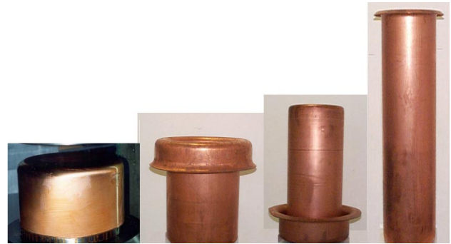
Fig. 7 - Reverse deep-drawing of seamless tubes. During each redrawing, the external surface of the cup to be drawn becomes the internal of the drawn part.
