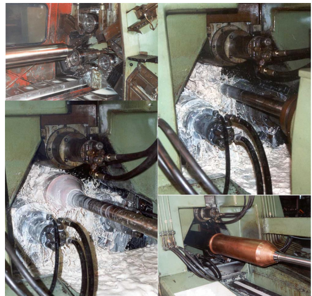
Fig. 8 - Forward flow-turning of seamless tubes. A short, thick tube is spun or drawn from a planar disk. Then the tube is thinned by three roller spinning.
