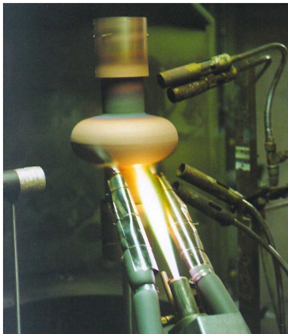
Figure 9: 1.3 GHz cavity performances before and after copper coating using the HVOF technique.
