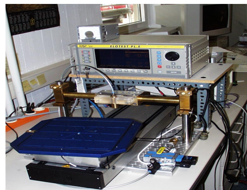
Fig.1 The eddy current scanning system
