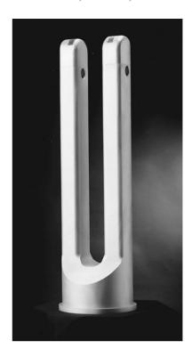
Figure 4: Half Wave Resonator for  $\beta_{opt} = 0.1$
