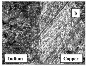
Figure 3: Stress lines and cracks in 60Sn/40Pb (a) and no developing of stress in indium-based solder (b) on copper sample after 10 thermal cycles in liquid nitrogen.
