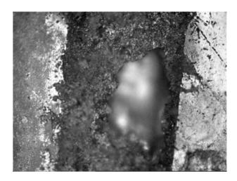
Figure 4: Etch of lead-tin solder on copper sample in CERN copper etch solution.
