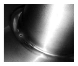
Figure 2: Photograph of cracks and exposed copper in electron-beam weld of resonator 304
