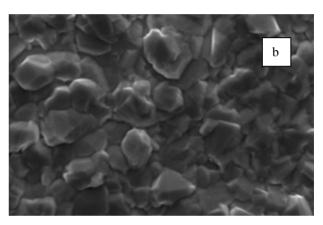
Figure 8: SEM images of lead-tin deposit electroplated onto silica wafer: a) film thickness d=2  $\mu$ ; and b) d=5  $\mu$ . A 0.3  $\mu$  copper layer was e-beam evaporated onto silica prior lead plating.
