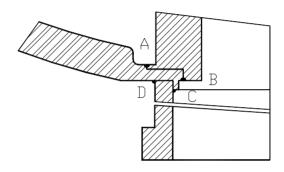
Figure 1: The electron-beam weld of the  $\beta$ =0.10 SLRs
