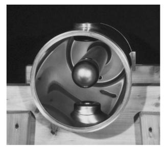
Fig.4. A medium  $\beta$  resonator obtained by Nb sputtered on Cu
