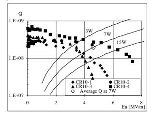
Figure 5: On line performance of Nb sputtered QWRs housed in cryostat CR10. The resonators are now working at an average field of 5 MV/m at 7W.
