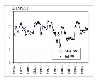
Figure 1: Performance of ALPI Pb/Cu resonators. They do not show any deterioration
