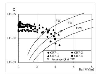
Figure 6: On line performance of Nb sputtered QWRs housed in cryostat CR7. The resonators are now working at an average field of 4.6 MV/m at 7W.
