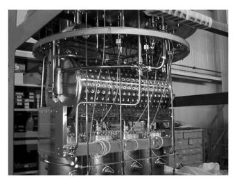
Figure 2. Upper flange of a low  $\beta$  ALPI cryostat. The cryogenic valve is on the top of the LHe reservoir
