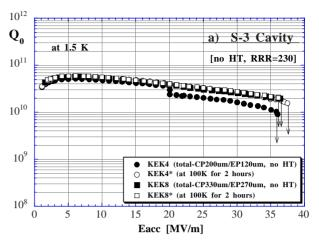
Figure 10-a): Effect of a 100K park in the S-3 cavity
