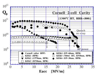
Figure 6: Test results in the Cornell two-cell cavity
