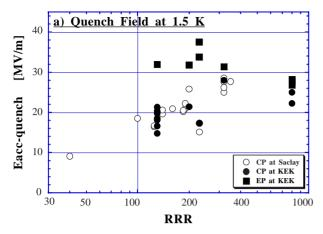
Figure 11-a): RRR dependence of the quench field (Six cavities tested at Saclay [3,17] are added in the data of CP at Saclay. A Saclay cavity with RRR=40 was made from reactor grade niobium. Test results on a KEK cavity with RRR=130 are shown in detail in reference [18].)
