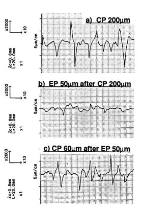
Figure 9: Surface roughness at the region thermally influenced by an electron beam in niobium samples.
