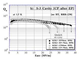
Figure 4-b): Cavity degradation due to CP after EP
