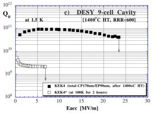
Figure 10-c): Effect of a 100K park in the DESY cavity
