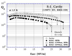
Figure 2: Test results in the S-1 cavity
