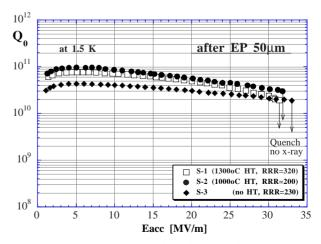
Figure 5: Three cavities after EP of 50µm
