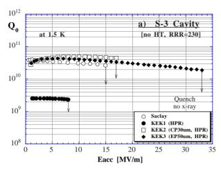
Figure 4-a): Test results in the S-3 cavity
