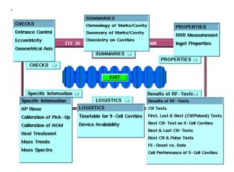
Fig.5: Start window of the cavity-related part of the GUI. By pressing the appropriate buttons windows are opened which contain for instance information as displayed in Figs.6 - 12.
