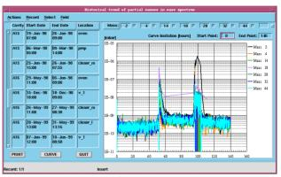
Fig.7: Historical trend of partial masses in mass spectrum during heat treatment of the cavity from "SPECIFIC INFORMATION". The time interval and the partial masses can be selected by the operator.
