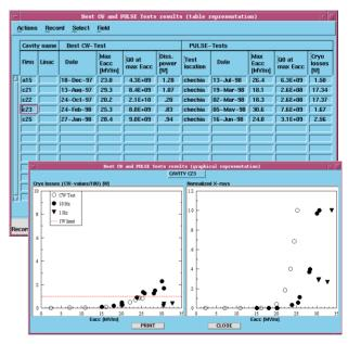
Fig.4: Comparison of CW and pulse test results for cavities installed in module 2 in table and graphical representation from "MEASUREMENTS" in Fig.3.
