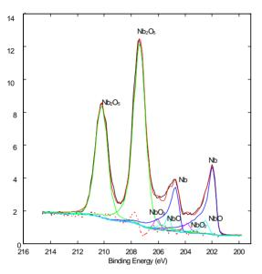
Figure 1 Deconvolution of the Nb3d line for one of the samples exposed to air; to reproduce the line-shape four chemical states (Nb, NbO, NbO<sub>3</sub>, Nb<sub>2</sub>O<sub>5</sub>) are necessary.
