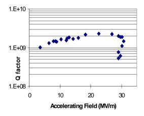
Figure 10: plot of Q factor vs. accelerating field after dry oxidation and HPP treatment.
