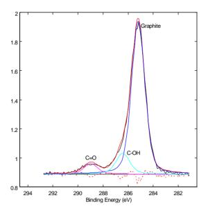
Figure 4 Deconvolution of the C1s line for one of the samples exposed to air; from the curve fitting we determine the presence of three chemical states (graphite, C-OH, C=O).
