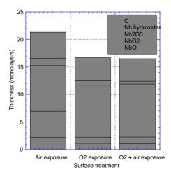
Figure 5 In-depth chemical composition of the samples exposed to air and to dry  $O_2$  (up to saturation). The last bar represents the in-depth composition of the dry oxidised samples exposed for a long time (about 10 days) to air after the dry  $O_2$  exposure. The errors on the thickness values are between  $\pm 0.1$  and  $\pm 0.3$  monolayers.
