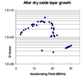
Figure 9: plot of Q factor vs. accelerating field after dry oxidation; the data in the right part of the plot were obtained during HPP treatment.
