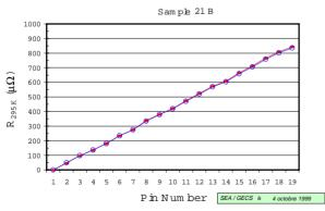
Figure 3 - Room Temperature Measurements. As expected, the resistance is linear with distance.
