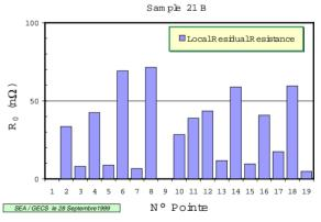
Figure 5 - Local measured residual resistance. Note that the value may vary by more than one order of magnitude from one place to another.
