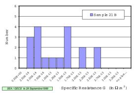
Figure 8 - Histogram of the specific resistance of grain boundaries in one sample.
