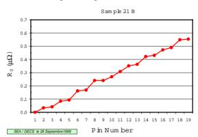
Figure 4 - Integrated residual resistance measured on a niobium sample. The result clearly shows a non uniform RRR.
