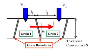
Figure 1 - Principle of grain boundary measurement.
