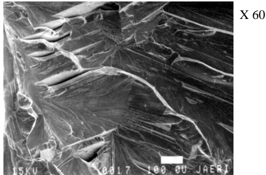
Figure 12: Cleavage fracture surface of sample No.3
