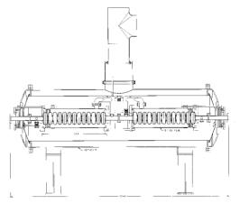
Figure 5: Cryostat module with two cavities.
