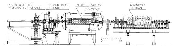
Figure 1: Elevation view of the photoinjector showing the gun, superconducting cavity and chicane.
