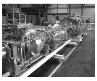
Figure 7: The two cavities in their helium tank and tuning systems before insertion into the vacuum vessel.
