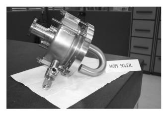
Figure 5: HOM coupler for dipole modes.
