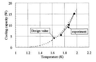
Figure 5:Cooling capacity of 1.8K line
