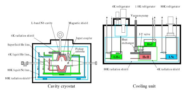
Figure 3: Schematic graph of the cryomodule
