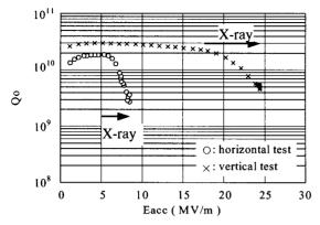
Figure 6: Quality factor as a function of accelerating field
