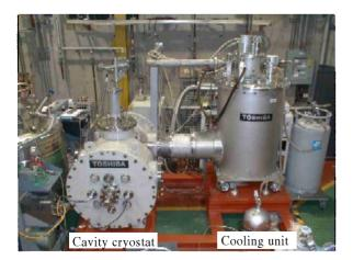
Figure 1: Cryomodule in a cooling test
