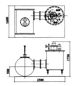
Figure 2: Dimensions(mm) of the cryomodule
