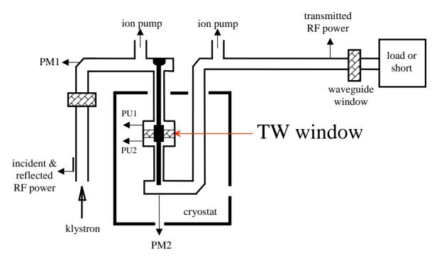
Figure 5: Schematic of test stand showing instrumentation
