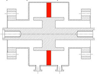
Figure 1: Sketch of the travelling wave window
