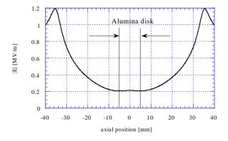
Figure 2: Electric field envelope in the ceramic disk region for 1 MW incident power
