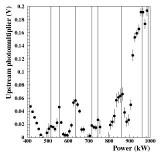
Figure 11: Upstream PM signal with smoothly varying component subtracted, showing multipactor barriers.
