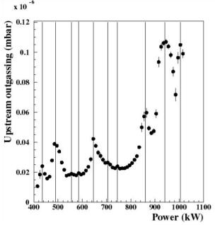
Figure 12 : Upstream outgassing signal, showing multipactor barriers.
