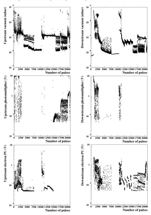
Figure 8 : Vacuum, photomultiplier and electron signals during the first conditioning. Upstream signals are on the left, downstream on the right.
