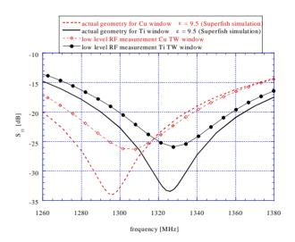
Figure 3: Measured and simulated  $S_{11}$  curve around 1.3 GHz.
