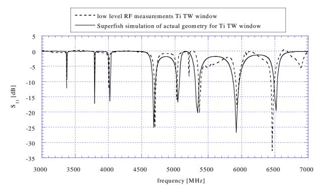
Figure 4: Comparison between the measured and simulated S<sub>11</sub> curve of the titanium window between 3 and 7 GHz
