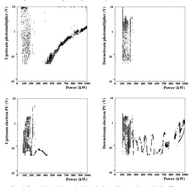
Figure 9 : Photomultiplier and electron signals during the first conditioning as a function of incident RF power.
