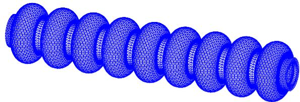
Figure 1: TESLA cavities with welded stiffening ring
