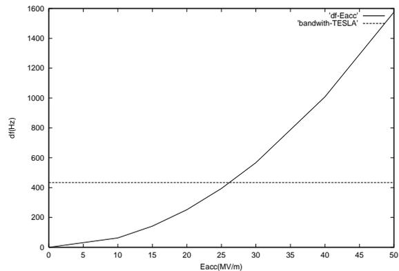
Figure 4: Bandwidth and frequency shift versus accelerator field
