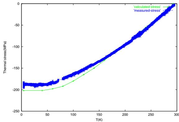
Figure 11: Stress at inner Nb surface
