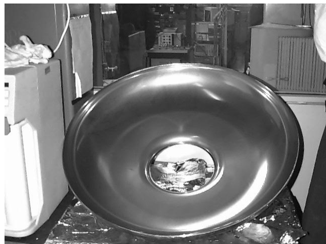
Figure 1; half of the Single cell cavity ready for the ESCA AUGER Measurements at the Genoa Lab
