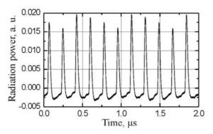
Figure 6: The output radiation time dependence. Electron bunch repetition rate 1.4 MHz is four time less then the optical resonator round-trip frequency 5.6 MHz.
