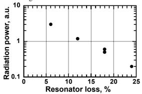
Figure 7: Average intra-cavity power vs. loss per one amplification.
