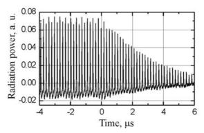
Figure 5: Time dependence of the output radiation power after switching the electron beam off.
