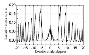
Figure 4: Results of the Fabri-Perot interferometer rotation angle scanning (radiation wavelength is 136µm).
