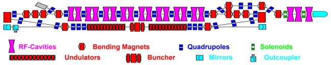
Figure 2: Scheme of the first stage of the Novosibirsk high power FEL.
