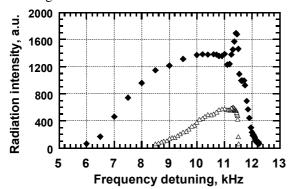
Figure 3: Laser intensity vs. RF frequency detuning f - 180400 kHz (diamonds at repetition rate 5.6 MHz, triangles at repetition rate 2.8 MHz).
