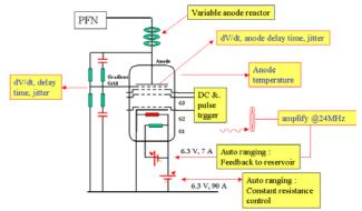
Figure 3: Experimental setup for the thyratron R&D.
