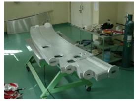
Figure 4: Welded dipole vacuum chamber
