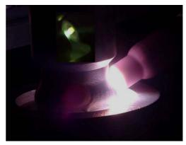
Figure 1: Welding of BPM port
