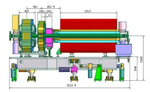
Figure 5: The magnets mounted on a girder.
