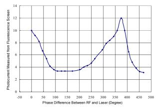
Figure 7: Electron beam current vs. phase difference between RF and laser.
