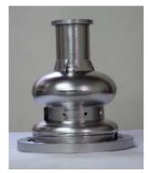
Figure 4: Image of the 1+1/2 cell niobium cavity.
