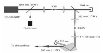
Figure 5: Optical scheme of the current drive laser.
