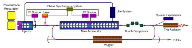
Figure 1: Schematic Layout of PKU-FEL facility
