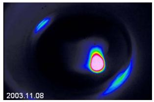
Figure 6: Beam spot at fluorescence, about 2 m apart from the photocathode.
