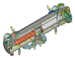
Figure 8: ELBE Module with two TESLA-type cavities in one cryostat
