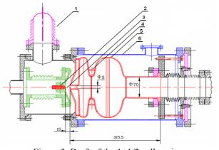
Figure 3: Draft of the 1+1/2 cell cavity. (1) Ceramic insulation (2) Photocathode (3) Pierce DC gun (4) Stiffening ring (5) Niobium cavity (6) LHe tank The structure of DC-SC injector has several advantages [2]:
