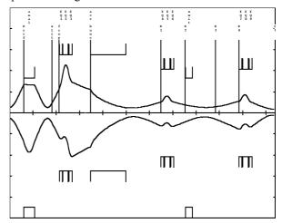
Figure 3: Beam envelope from ECR source upto RFQ entrance
