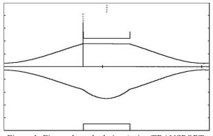
Figure 1: First order calculation (using TRANSPORT, upper: non- dispersive plane, lower: dispersive plane)
