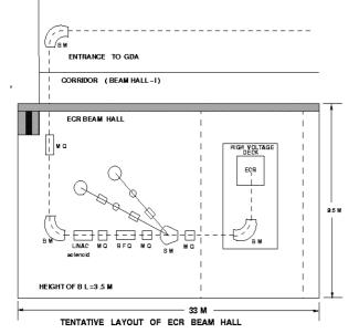
Figure 5: Layout of beam hall for the high current injection into superconducting linac
