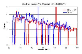
Figure 5: The hadron events rate vs. beam current in the parasitic mode and normal colliding mode.
