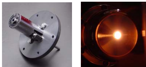
Figure 1: CeB 6 cathode assembly.
