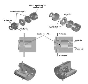
Fig. 4: Construction Schematic view of Nb target
