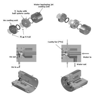
Fig. 1: Construction schematic view of Ti target
