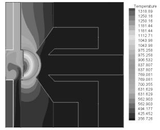
Fig. 2: Temperature contour of target(12.5 MeV, 50 µA)
