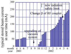
Figure 3: Increase of the typical stored beam current during the user time.
