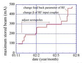
Figure 4: Improvement of the maximum stored beam current. The maximum current was limited to 500mA by the radiation safety condition at the present.
