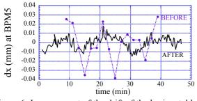
Figure 6: Improvement of the drift of the horizontal beam position by the stabilization of the cooling water temperature from  $\pm 1.5$  degrees to  $\pm 0.5$  degrees. The BPM15 is one of beam position monitors set at the dispersive sections.
