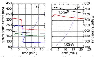
Figure 5: The stored beam current with the tuning angle of  $-5^{\circ}$  (left plot) and  $-21^{\circ}$  (right plot). The broken lines are current of bending magnet (right axis). The solid lines are examples of stored beam current (left axis) during the acceleration. The beam had been lost by the horizontal TM110 HOM.
