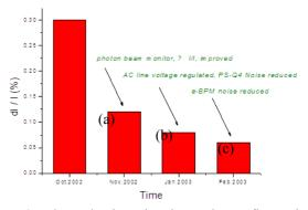
Figure 3: The reductions in photon beam fluctuations. Improvements of  $I_0$  monitor (a), ripples reduction in Q4 power supply (b), and in electron BPMs (c).
