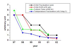
Figure 2: The improvements in reliability, temperature fluctuation and beam orbit stability at TLS.
