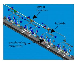
Figure 3: Phase 2 distribution circuit.
