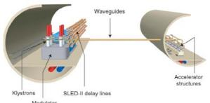
Figure 1: X-band linear collider two-tunnel layout, showing overlapping SLED-II delay lines, klystrons sharing a modulator, and a waveguide system transporting and distributing power to a set of accelerating structures.
