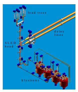
Figure 2: Phase 1 layout showing klystrons and the dual-moded SLED-II pulse compressor.
