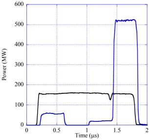
Figure 5: Peak power meter measurements of high power waveforms. The black trace is the input power and the blue trace is the output of the pulse compressor
