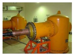
Figure 8: The high voltage accelerator developed in SINAP for EB cleaning flue gases.
