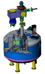
Figure 6: Main structure of CYCIAE-10.
