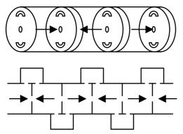
Figure 1: Accelerating structures used in medical SW linacs, magnetic on-axis coupled (up) and side-coupled (down).
