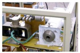
Figure 10: The X-band travelling wave mini linac by Nanjing University.
