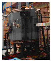
Figure 7: The 10MeV cyclotron developed in LIMP.
