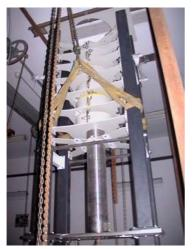
Figure 9: The 10MeV radiation processing travelling wave accelerating waveguide.
