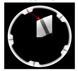
Figure 11: The CT space resolution testing picture by a ICT system with a 9MeV SW linac by CAEP.
