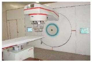
Figure 3: Photo of the 16MeV travelling-wave electron linac HM-J-16.
