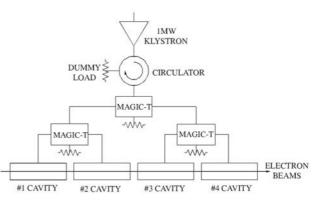
Figure 1: Original rf system of the PF-AR west rf station.
