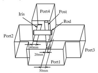
Figure 3: Structure of asymmetric power divider.
