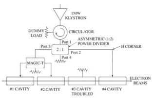
Figure 2: Modified rf system for operating three cavities.
