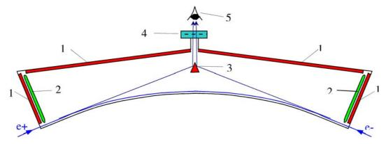
Figure 4. Bending magnet vacuum chamber. 1- Copper SR absorbers; 2- pumping holes to ion pumps; 3 - double sites morrow: 4 -window; 5 - beam profile monitor.
