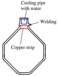
Figure 5. Cross-section of the straight vacuum chamber.
