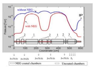
Figure 2: Pressure profile along quota of perimeter with and without NEG coating in the straight sections. 1 – bending magnet, 2 – quadrupole, sextupole lens, 3 – superconducting solenoid.
