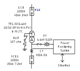
Figure 3: Power monitoring network diagram of 6.6 kV electric powers.
