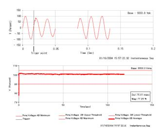
Figure 4: A sample graph captured at the instantaneous voltage sag.
