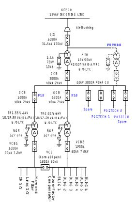
Figure 1: Single line diagram of the PLS AC power.
