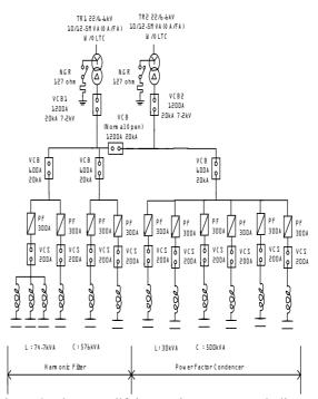
Figure 2: Phase modifying equipment network diagram
