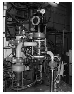
Figure 2: Electron beam system designed for conversion of silicon tetrachloride into trichlorosilane.
