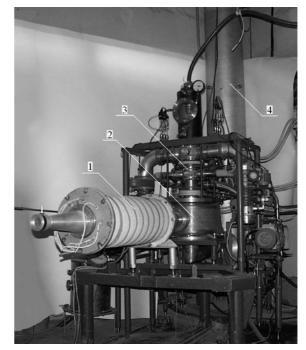
Figure 4: Experimental facility for gas cleaning of toxic impurities with the help of concentrated electron beam.
