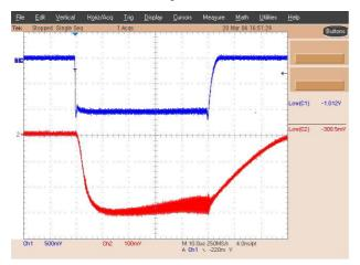
Figure 7: Pulse shape in high power test at 352.1MHz
