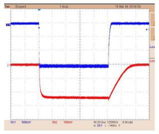
Figure 4: Pulse shape of the klystron at 350MHz
