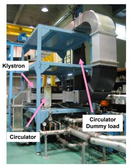
Figure 1: Klystron, circulator, dummy load
